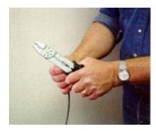
Loosen the nut on the strain relief attached to the terminal block cover.
