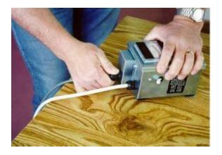
Remove the terminal block cover on the bottom of the KTA box by unscrewing the four sheet metal screws that hold it in place.
