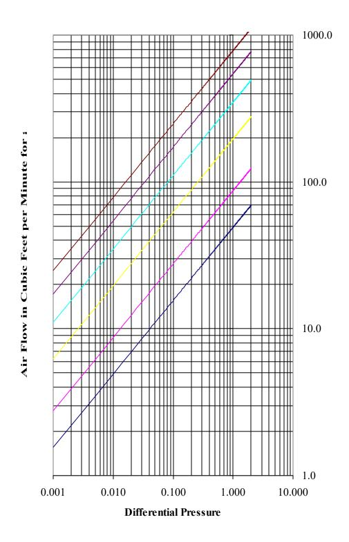
Example: A micromanometer reading of 0.019 in a 4inch pipe was obtained. The flow is  $48 \, \text{CFM}$
