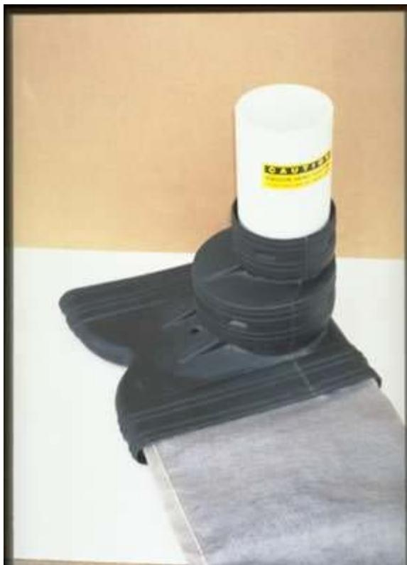
Slide the mat into either end of the riser and tape the edge to prevent wet concrete from entering.
