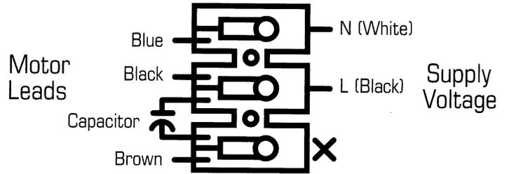
There are typically three wires to be connected to an electrical fan; Load, Neutral and Ground. Load provides power to the fan, Neutral is for returning current and closing the electrical circuit, and Ground is for an additional path to safely return current to the ground, in case of an accidental electrical short in the fan and/or discharging of fan metal components.
